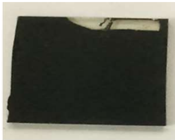
Figure 2(a): PbI 2 layer deposition on the FTO glass; (b): CH 3 NH 3 PbI 3 layer deposition on FTO glass.
