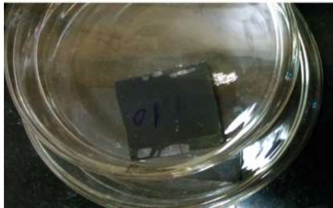
Figure 2(c): perovskite film in the desiccator
