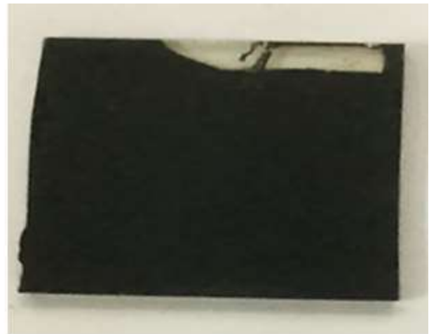
Figure 2(a): PbI 2 layer deposition on the FTO glass; (b): CH 3 NH 3 PbI 3 layer deposition on FTO glass.
